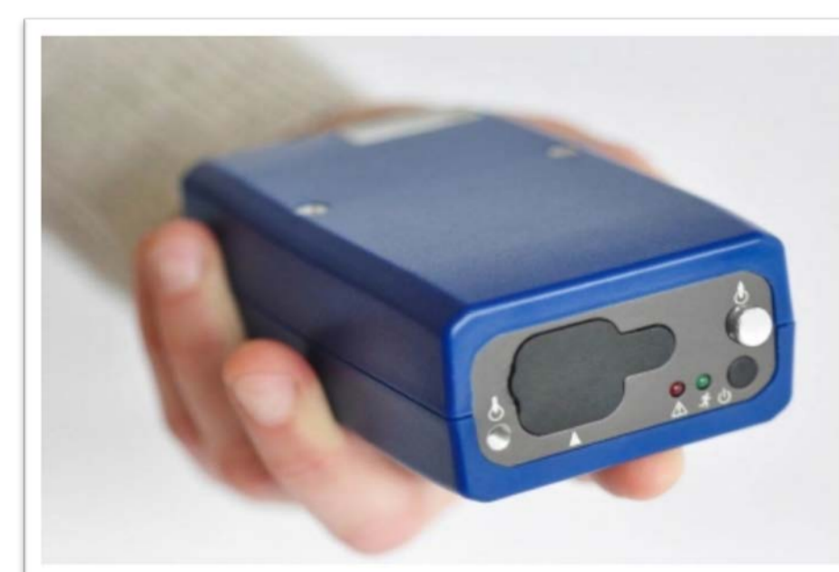
Figure 4: AE-51 Aethalometer – world's first real time, portable Black Carbon aerosol monitor. The measurement accuracy is of +/- 0.1 \mu\text{g Eq.C/m}^3 at 150 ml/min. Figure taken from Ecomasure (2015).
